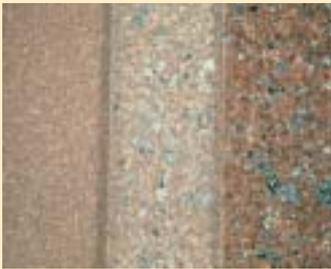
*The single concrete mix shown here has three different finishes. From left to right, they are acid etch, sandblast and retarded. This multiple-finish technique offers an economical, yet effective, way to heighten aesthetic interest.*
