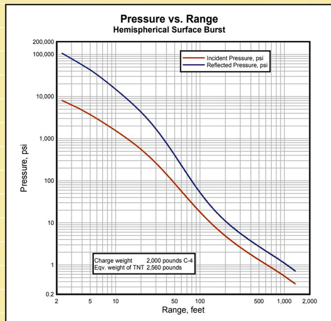
Fig. 6 – Pressure vs. Range-Hemispherical Surface Burst.\*
