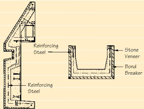
**Fig. 1 Typical spandrel and column cover panels.**
