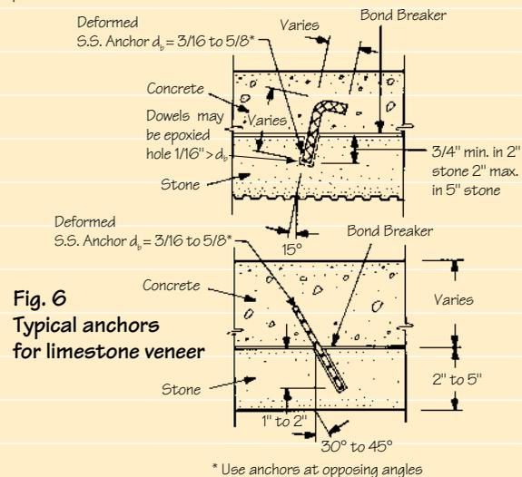
**Fig. 6 Typical anchors for limestone veneer**
