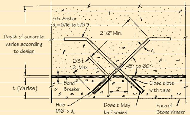
**Fig. 5 Typical cross anchor dowels for stone veneer**
